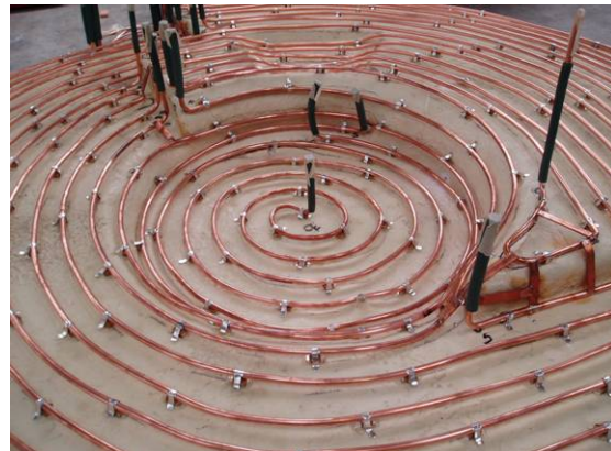
Fig. 8 (left) Carbon/epoxy helmet moulding produced from water temperature controlled mould; (right) series of copper temperature control pipes being installed on the rear face of a composite LRTM production mould.
