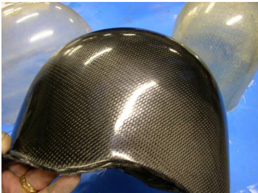
Fig. 8 (left) Carbon/epoxy helmet moulding produced from water temperature controlled mould; (right) series of copper temperature control pipes being installed on the rear face of a composite LRTM production mould.
