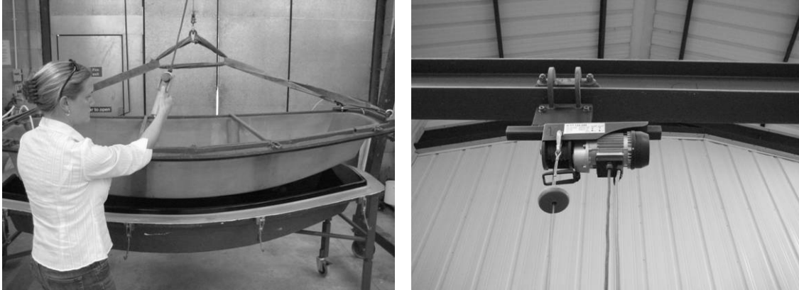
Fig 12 5 m 2 small boat mould being lifted with low cost industrial hoist.
